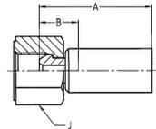
**MATERIALE** Galvanised steel with transparent Cr(VI)-free plating. For fittings as mentioned above, but with stainless steel nipple (AISI 303), please add **C2W** to the Part No. Example: 1U0NX-8-08 **C2W**. Other materials available on request.
